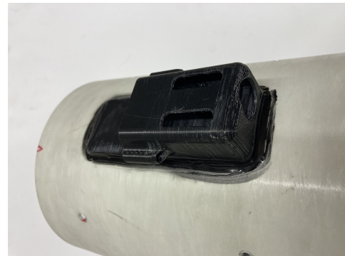
Figure 41: Camera shroud secured on payload bay
