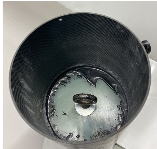
Figure 35: Fin Can Bulkhead epoxied into body tube
