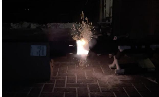
Figure 124: Drogue separation point ejection charge test
