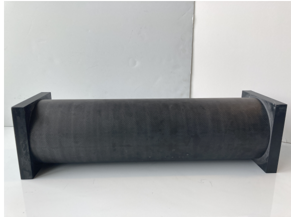
Figure 29: Body tube in CNC mounting jigs
