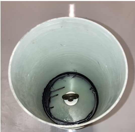
Figure 34: Payload Bulkhead epoxied into body tube
