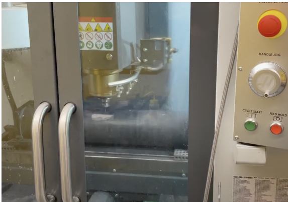
Figure 30: Body tube mounted in CNC mill
