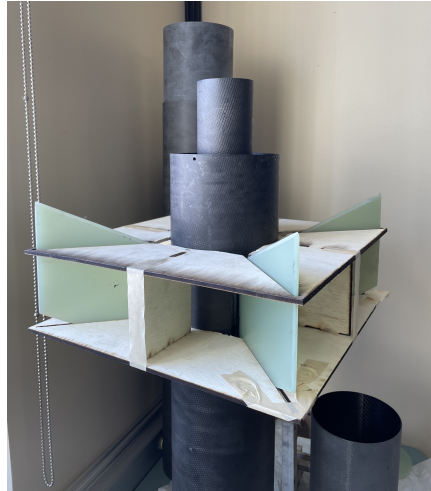
Figure 39: Fins held in place by wooden alignment jig
