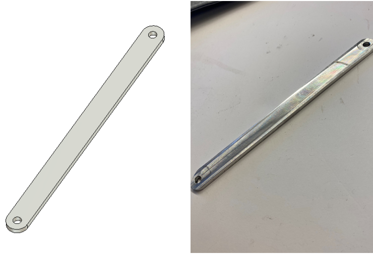
Figure 101: CAD model (left) and as constructed (right) Pusher Arm
