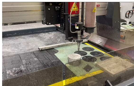
Figure 27: Image of waterjet cutting bulkheads and centering rings
