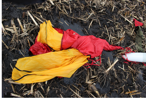
Figure 121: Tangled main parachute after landing
