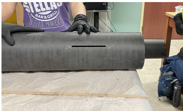
Figure 37: Motor Mount being secured in fin can
