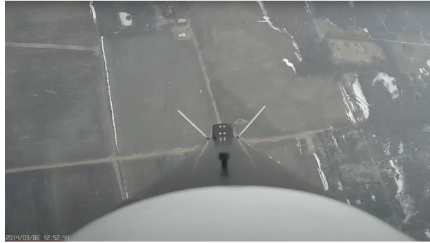
Figure 126: ACS flap actuation as seen from on-board camera
